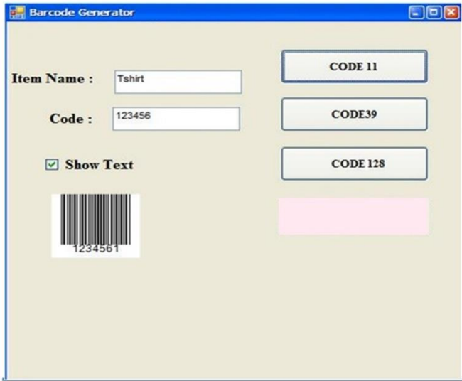
Figure 9 Barcode Creation with Code 11
