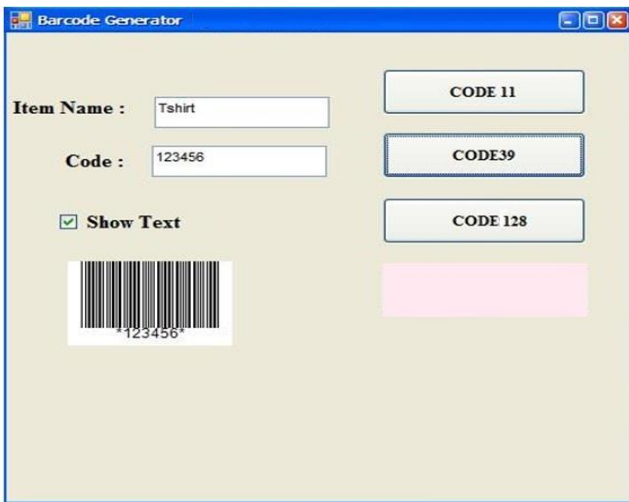
Figure 10 Barcode Creation with Code 39
