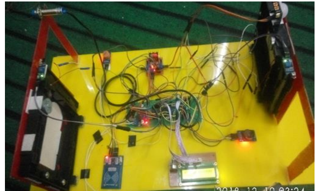
Figure 12. Final Assembly of Automatic Safety Entrance System
