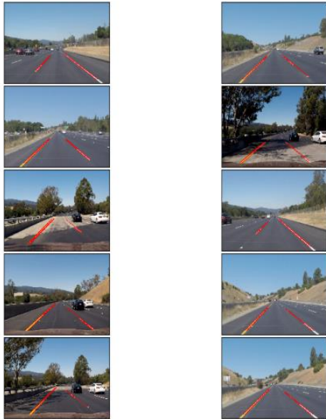
Figure 7. Simulation Result of Line Detected Images
