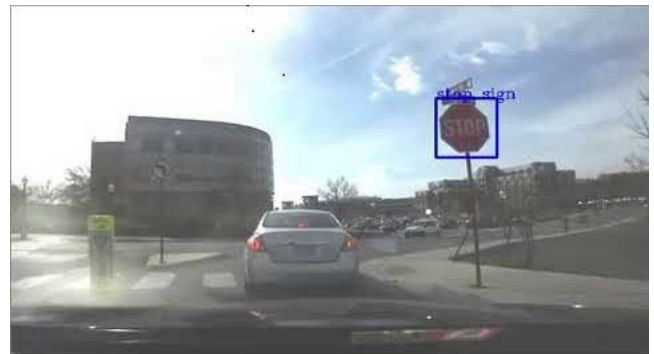
Figure 19. Result of Stop Sign Detection from Real-Time Video
