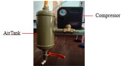
Figure 6. Design of Air Tank and Compressor
