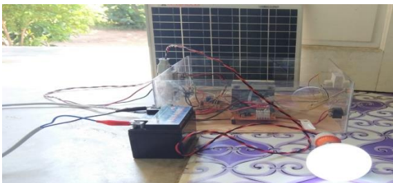
Fig 10: AC Load ON Condition
