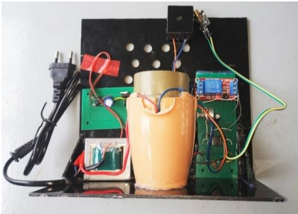
Figure 11. Internal Circuit of Automatic Hand Dryer
