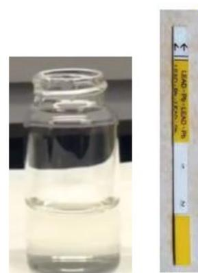
Figure IV. Treated water sample (Pb<sup>2+</sup> free).
