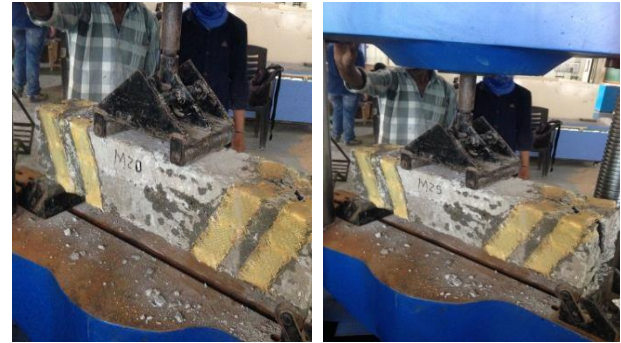
Fig 7 Four point loading for Shear test of 45° Degree Strip-wrapped Beam M20 & M25 (AFRP sheet)
