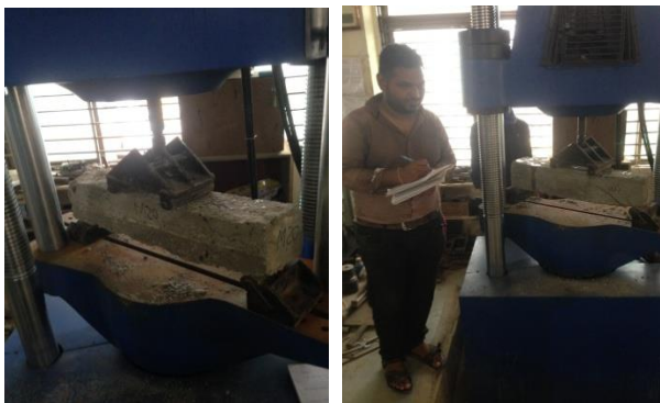
Fig 6 Four point loading Testing setup UTM and shear test of control specimen M20 & M25
