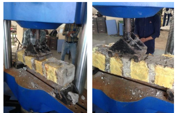
Fig 9 Four point loading for Shear Test of Vertical Strip-wrapped Beam M20 & M25 (AFRP sheet)
