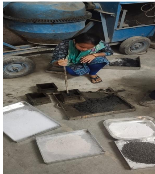
Casting of the cube
